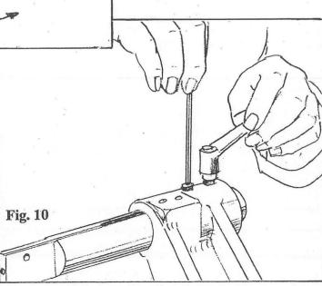
17. Using the M6 Bolts, flat washers and Nyloc Nuts, loosely fit the Handle Link (SBT 4) to the Handle Bracket. Then fit the Handle (SBT 5) to the Handle Link and then connect the Handle so that it sits over the flats machined on the rear of the Tailstock Quill. (Fig. 11)
