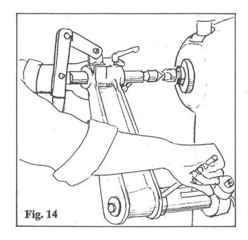
24. When tightening the Taper Clamp Cap Screw that retains and locks the Tailstock Body Casting on its eccentric mounting taper, it will be necessary to apply counterpressure to the casting to prevent it moving with the twisting pressure of the Taper Clamp Cap. Do this by applying anti-clockwise force to the top of the Tailstock Body Casting as the clamp screw is tightened. Check continually that the alignment of the centres is maintained. (Fig. 15)
